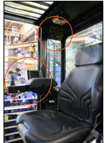
Controls and gauges are located out of the way, but easily within operator's reach.
