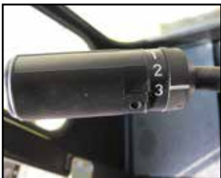
Directional/gear-shift lever on steering column
