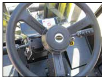
In addition to the tilt steering column and air ride seat, the "dashless" design provides more legroom and easier entry/exit for the operator for superior ergonomics and comfort
