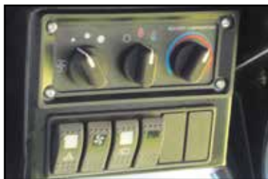
Cab heater with defroster and fan. Optional air conditioning unit available.
