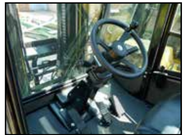
"Dashless" cab provides more space and visibility for the operator; Eliminates incidental damage to gauges and controls previously located on the dashboard
