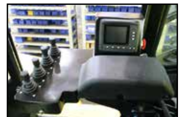
MD3 display, located on the armrest with fingertip hydraulic controls, provides digital gauges for water temperature, fuel level and oil pressure. Other features include tachometer, battery indicator, parking brake indicator and RemoteTech warning/service messages.
